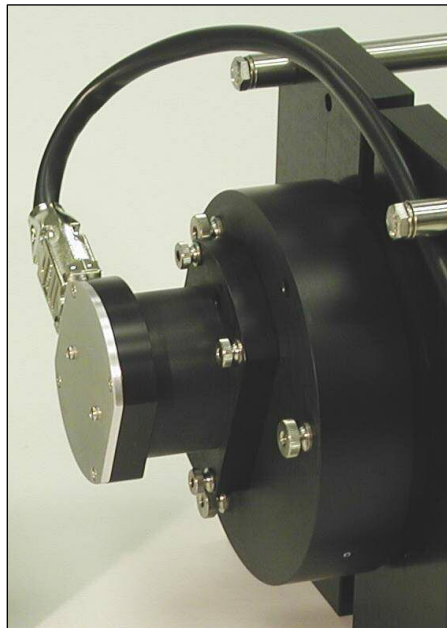
Figure 7 SLS head mounted on HydroRad-ES1
