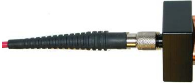
SMA cable attached to radiance collector. For underwater operation the SMA connection must be sealed.
